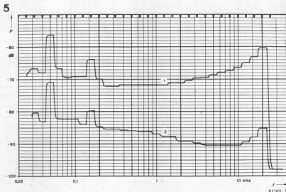
Figure 5. The noise spectrum characteristics of a cassette tape without compander (1) and with High Com (2).
