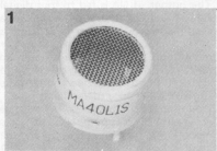
Photo 1. This is what a typical transducer looks like. Note that two different types are used in the transmitter and in the receiver.
