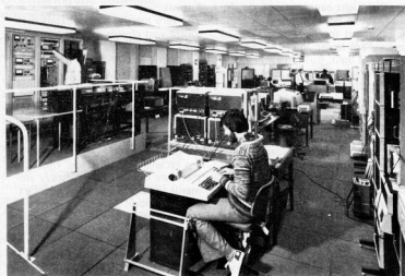
IRAS control centre at RAL, responsible for monitoring the status of the satellite and collecting data from its primary telescope and other experiments. The satellite passes over the centre at least twice daily. Incoming data gives scientists a brief check on objects that have been observed and controllers can make checks on the spacecraft itself. Data is sent to the Jet Propulsion Laboratory for complete processing.
