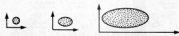
Figure 2. Because large raindrops become distorted as they fall, they give a lot more back-scatter from horizontally polarised waves than they do from waves with vertical polarisation, whereas small drops, remaining almost spherical, back-scatter both types of wave in sensibly equal amounts.
