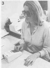
Figure 3. This electronic calculator enables the blind to benefit from modern technology by displaying the figures in braille.
