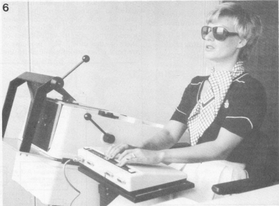
Figure 6. This reading device will convert any text into braille.
