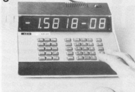
Figure 5. The calculator for myopic operators reproduces figures that are four times the size of those shown on ordinary calculators.
