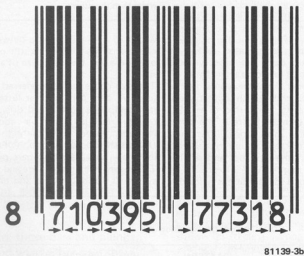
Figure 3. Two examples of product coding. Bars and spaces may have four different widths. Two bars and two spaces make up a single digit. In figure 3a digits (0 and 4) have been added to enable errors to be detected in the main block. In the right-hand block this is done by changing the write direction of the digits. In figure 3b the write direction is used to detect errors throughout the block.
