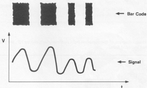
Figure 3. Two examples of the type of signals that the sensor is likely to produce. Figure 3a shows a fairly good print sample and figure 3b illustrates what can go wrong.
