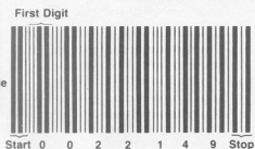
Figure 1. In the 'two out of five' code one digit is represented by five bars, two of which are wider than the others.
