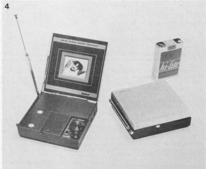
Photo 4. Liquid crystal screen in a pocket TV prototype manufactured by National Panasonic (Matsushita). With a total of 57,000 display dots it operates on a supply of 4.6 V.
