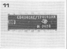
Figure 11. Texas Instruments CMOS IC. This IC carries two type numbers! One type number prefixed 'CD' is identical to that used by RCA, the other is prefixed 'TP'. Suffix 'A' for A-series unbuffered or 'B' for B-series buffered. Package suffix is 'N' for plastic or 'J' for ceramic.
