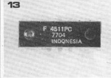
Figure 13. A Fairchild CMOS IC. Type numbers of Fairchild CMOS devices are prefixed by 'F' and sometimes by '3'. All Fairchild ICs are buffered except where the circuit configuration makes this impossible. Package suffix 'P' for plastic or 'D' for ceramic, followed by 'C' for commercial temperature range or 'M' for military temperature range.
