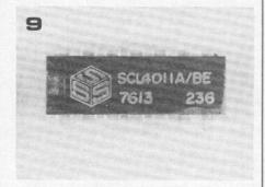
Figure 9. Solid State Scientific CMOS IC. Prefix 'SCL', suffix 'A' for A-series unbuffered, 'A/B' for A-series buffered, 'UB' for B-series unbuffered and 'B' for B-series buffered. This is followed by 'E' for plastic package or 'D' for ceramic package. Maximum supply voltage of all SSS CMOS ICs is 18 V.
