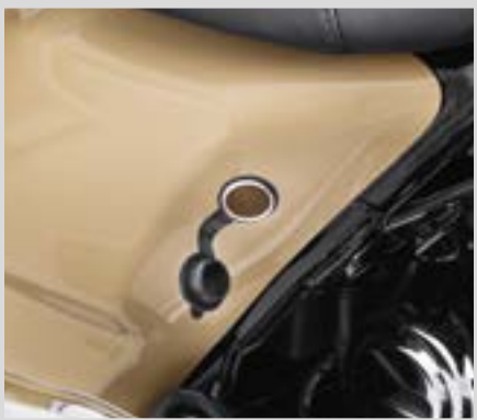
G. AUXILIARY POWER PORT – SIDE-PANEL MOUNT
