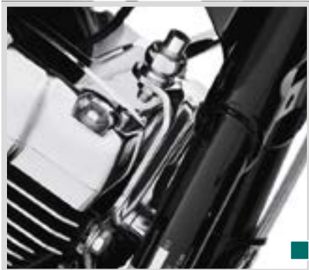
G. FRONT ENGINE MOUNT STABILIZER LINK
