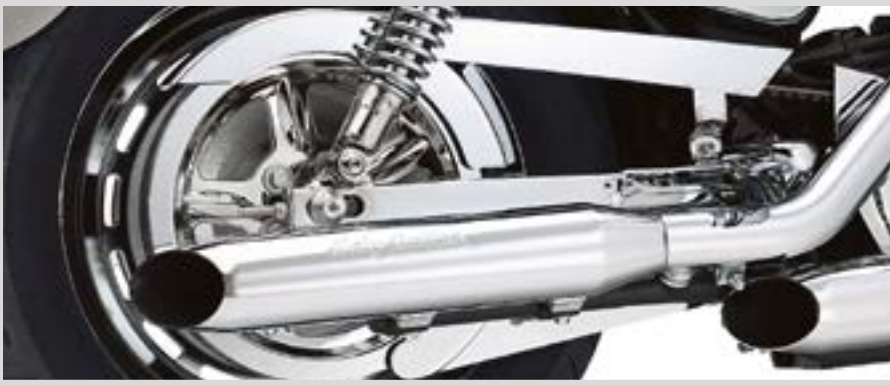
F. UPPER BELT GUARD – CHROME (SHOWN WITH CHROME LOWER BELT GUARD AND SWINGARM)
