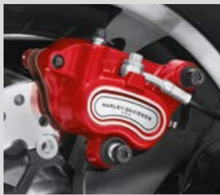
H. BRAKE CALIPER KIT – RED (41300157 SHOWN)
