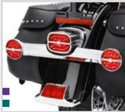
A. LED FLAT LENS TURN SIGNAL – RED
