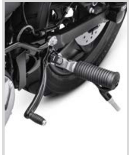
A. REAR SET FOOT CONTROLS – SPORTSTER MODELS
