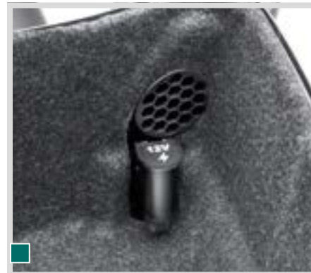
E. AUXILIARY POWER PORT – TOUR-PAK MOUNT '14-LATER MODELS
