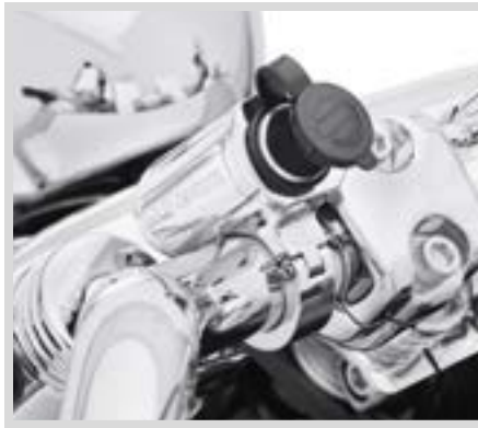
A. AUXILIARY POWER PORT – HANDLEBAR MOUNT – CHROME
