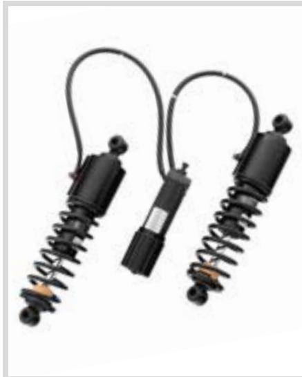
H. PREMIUM RIDE HAND-ADJUSTABLE SHOCKS – TRIKE MODELS
