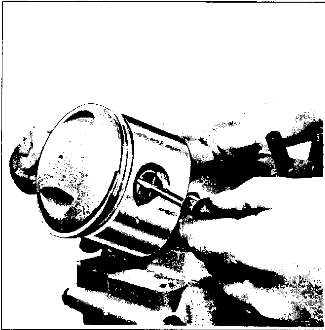
Figure 3C-2. Removing Piston Pin Lock Ring
