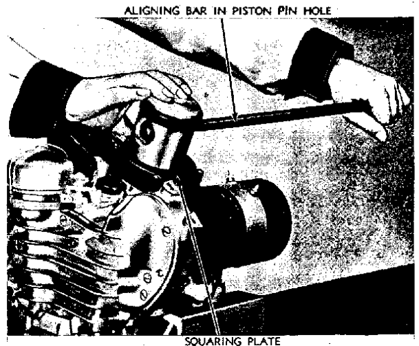
ILLUS. 71 STRAIGHTENING BENT OR TWISTED CONNECTING ROD
